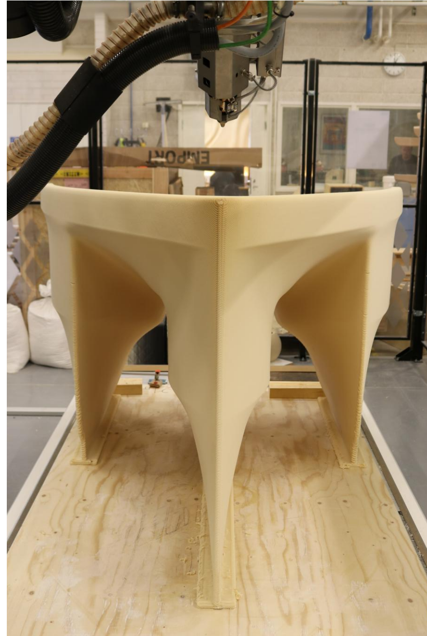
3D-printed hull of a trimaran
